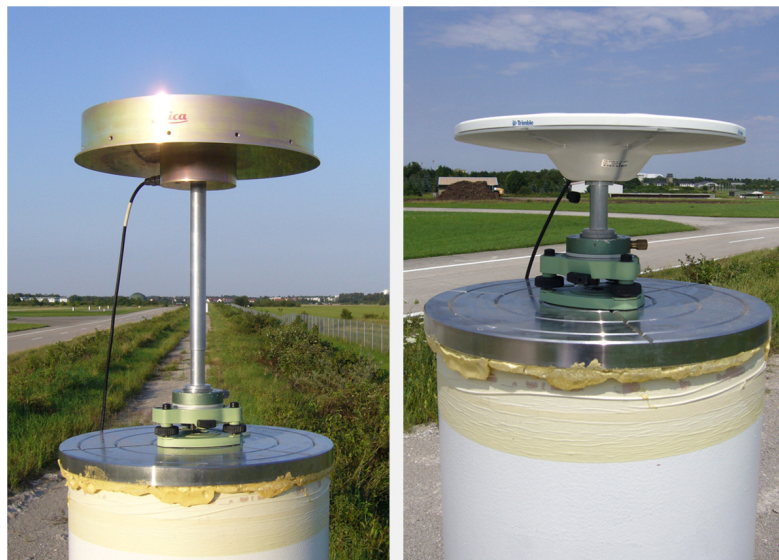
Fig. 4: Pillars and antenna mounting
