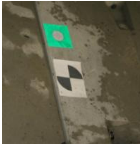
Figure 6: Trimble Target (Upper example) - Leica Target (Lower example) (Source: A. De Wulf, 2009)
