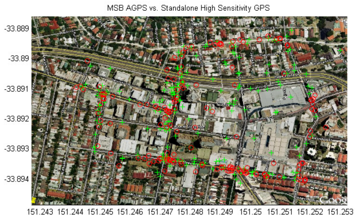
Figure 3. A-GPS (green cross) and standalone high sensitivity GPS (red circle) positioning results.
