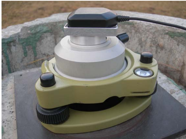
Figure 3: Constructed adapter for the u-blox antenna
