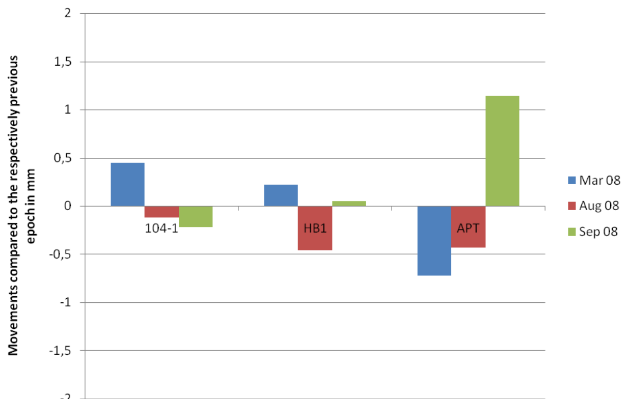
Figure 9: Deformation analysis results for the levelling to the anchorage point
