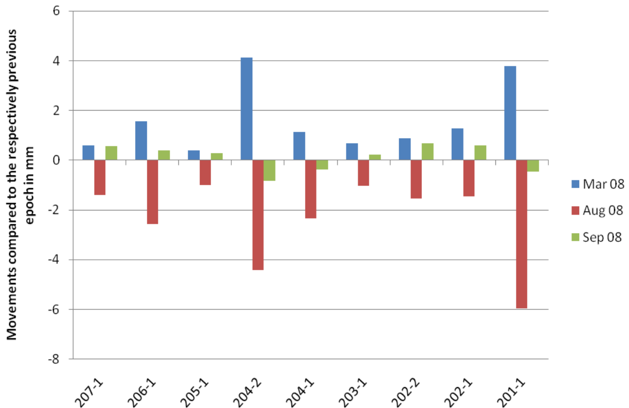
Figure 11: Deformation analysis results for the upper street
