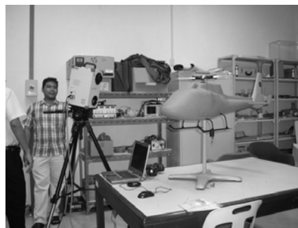
Figure 12: Laser Scanning set-up
