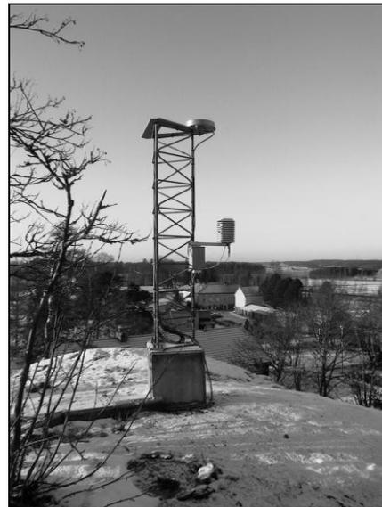
**Figure 3.** A mast of Tuorla permanent GPS station. This kind of a 2.5 m height steel grid mast is a typical antenna platform at FinnRef GPS sites.
