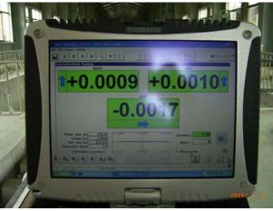
**Fig.3.16** Post-Adjustment Measurement. Difference from design is less than 2mm. Green indicates pass; yellow indicates over.
