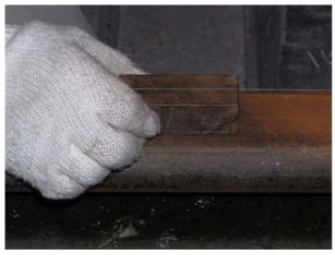
Fig.3.7 Setup of Measurement Device for Conventional Positioning Elevation Survey at the Measurement End
