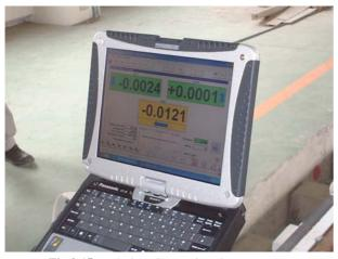
**Fig.3.15** Real Time Comparison between Coordinates of Station Survey and Design Lineshape for Adjustment.
