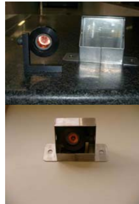
Figure 5 Mini Prism with protective shield
