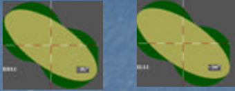
The error ellipses on the southern tunnel portal
