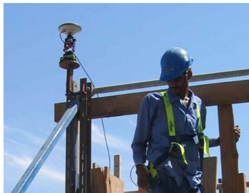
Figure 1: GPS and circular prism collocated
