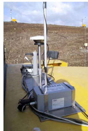
Sensor on top of compactor
