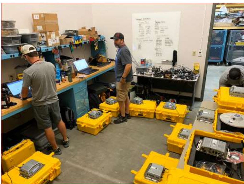
Figure 6: NGS personnel configure receivers prior to the IGLD 2020 campaign
