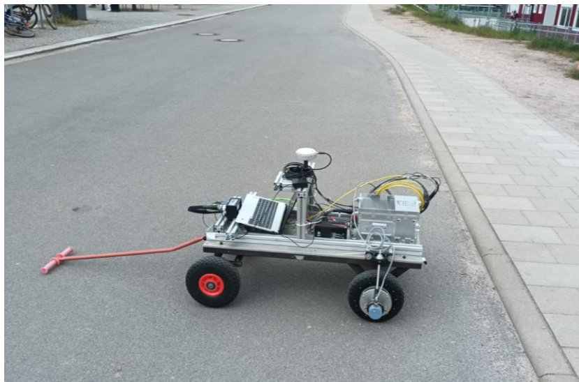
Figure 7: Hand cart with test setup and RLG-IMU as ground truth; the curb you can see is used as a pipeline replacement
