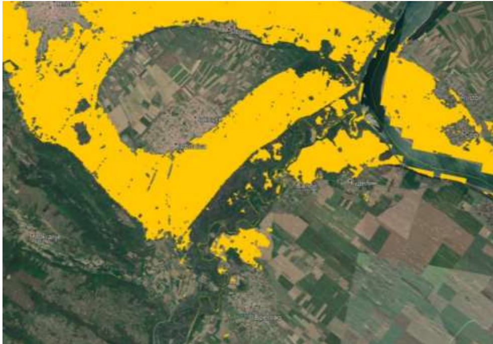
Figure 7. Flooded areas as detected by SAR from descending orbit on March 6 th 2018 when the flood is at its peak.
