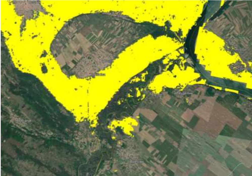
Figure 8. Flooded areas as detected by SAR from ascending orbit March 07 th 2018 when the flood is at its peak.
