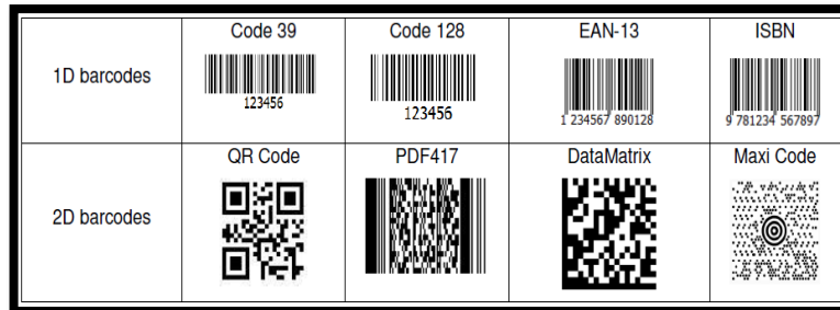
Figure 3: The types of 1D and 2D barcode (Jun et al., 2010)
