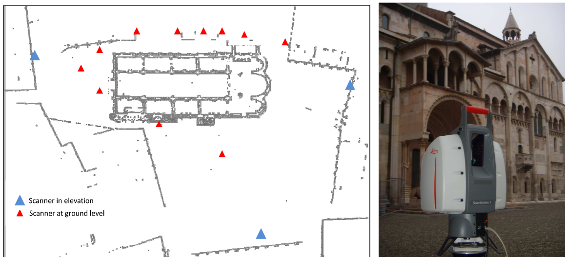
Figure 3. Surveying the Cathedral of Modena: design of the external laser scanner positions (left); the laser scanner while operating (right).
