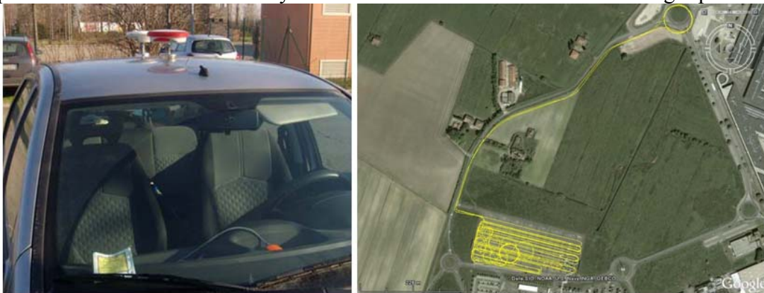
Figure 6. Test configuration: vehicle equipment with both GPS on the top and the magnetometer inside (left side); comprehensive view of the area with trajectories (right side).
