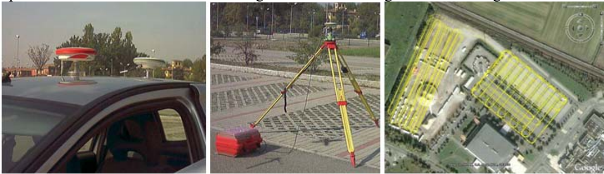
Figure 1. Test configuration: the vehicle equipment with both GPS on the top (left side), the master station for the reference solution processing (middle) and the trajectories (right side).
