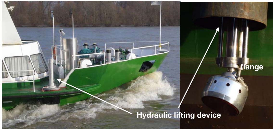
Figure 5: transducer mounting and bow waves
